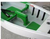
Centre Board Bungee. This is the shock cord that is "woven" around the dagger board trunk. Check rope is in good condition and "weave" configuration suitable. If shock chord is spent the centre board won't stay in position.
