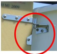
Particularly check your pintels and Gudgeons- they bend and result in rudders "popping" out. Sometimes you can straighten them out with pliers. Replacement of bents ones is a good plan. Make sure the retaining clip works and keeps the rudder on.
